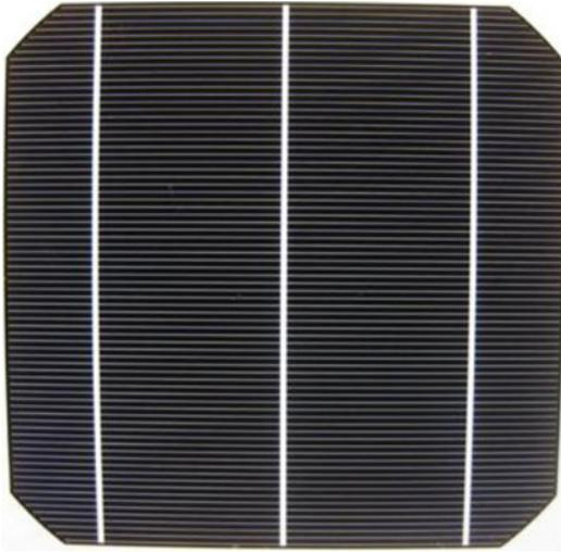
Fig. 3. Photograph of 156-mm pseudosquare cell with grid pattern of the type analyzed.
